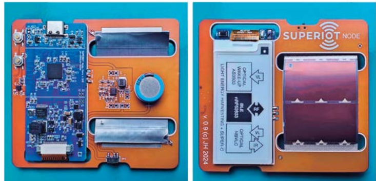
SUPERIOT reference radio-optical IoT node with light-based energy harvesting
